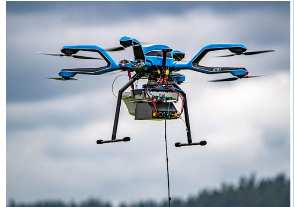
Image: Cell on Wings (COW) Weather Hardened UAV. Image Source: AT&T, 2018.
