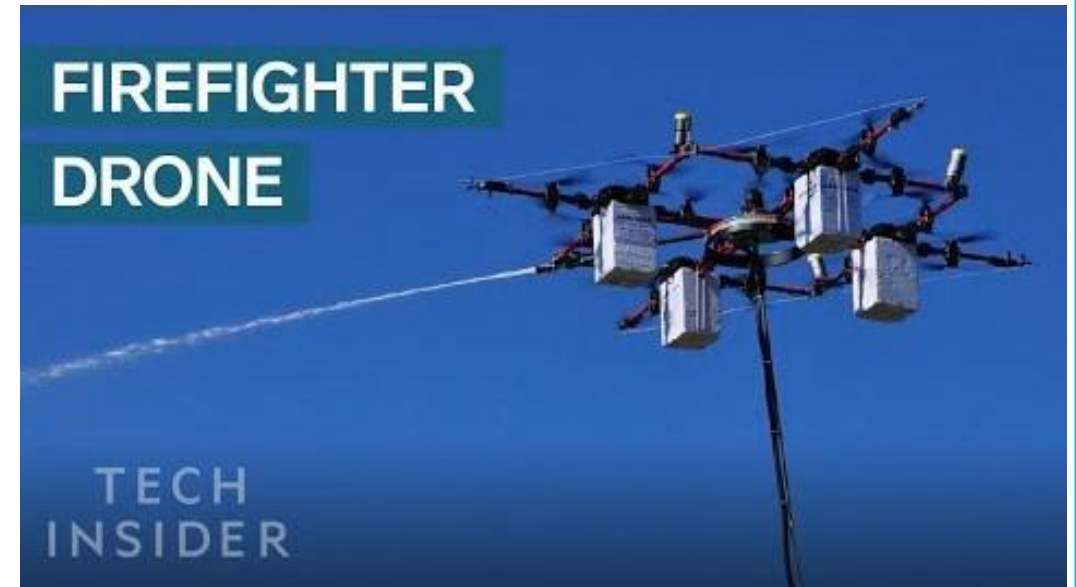
Video: Aeronne firefighting UAV demonstration. Image Source: Aerones, 2019.
