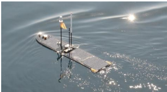
Image: Lyra autonomous 'Wave Glider' vehicle used to monitor fish stocks. Image Source: Cefas, 2018. http://bit.ly/35ROWwa .
