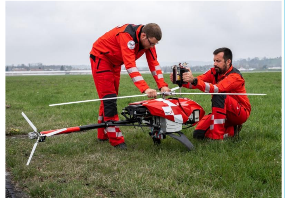
Image: The Rega Search and Rescue Drone, which operates autonomously and can search for victims over a several kilometers for several hours at a time. Image David Neld, 2019. http://bit.ly/2JfitGI .
