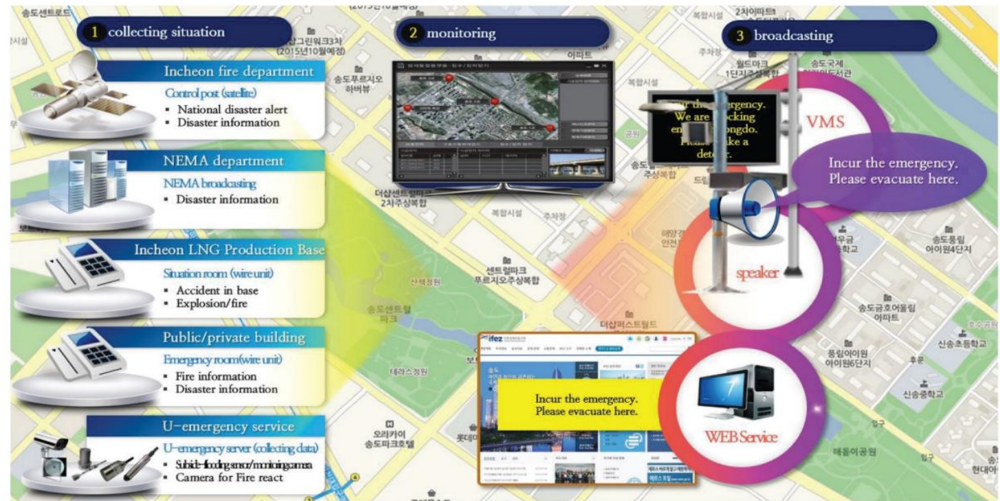
Image: Diagram of emergency response services provided by Songdo Smart City system. Image credit: IDB-KRIS, 2016.
